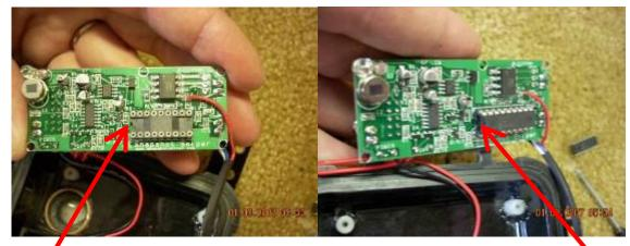
Note the notch on the end of the Socket.
