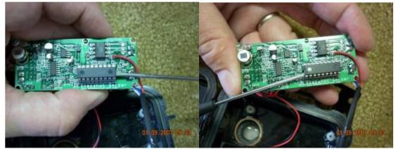
Gently pry on each end of the existing chip to remove it from the socket.
