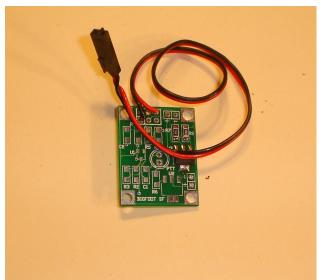
The Slave board comes pre wired with a connector that will plug directly into the Bigfoot sensor board. The Bigfoot board will need to have the slave program in the microcontroller to operate your slave properly.
