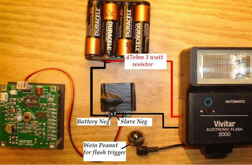
This allows a very simple connection of your slave to the Bigfoot sensor. The slave board allows the Bigfoot sensor and its day night circuit to control the charge circuit of the slave flash making it a very reliable and efficient slave. The Wein peanut is the best option at this point for the flashes trigger. <u>As precaution I recommend that the slave's flash capacitor be drained before you connect or disconnect the Wein Peanut to the sync cord.</u>
