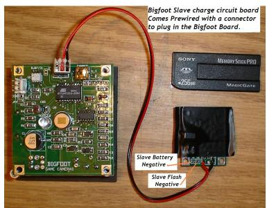
The Slave board connector will be plugged into the top row of pins on the header with the wires coming out away from the Bigfoot board.
