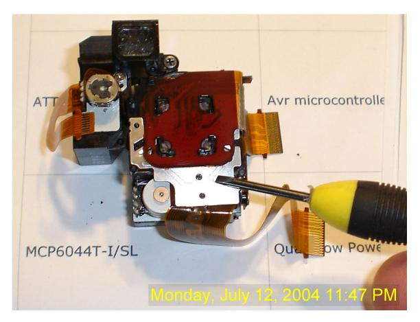
Now you will see the CCd ribbon The CCd is attached directly to this ribbon on the opposite side. It is held in place with 4 sonic welds there also is a small screw holding it on the right side. Remove that screw also.
