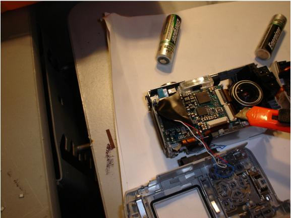
Once the 3 cables are disconnected the whole lenses assembly will lift out It's a little tricky here but I just lift it by the plastic of the viewfinder and it will sort of snap out. Again lay it faces Lenses side down on a clean soft rag.
