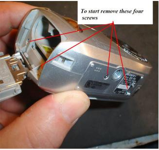
To open the camera 4 screws must be removed
