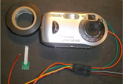
The first thing I will do with either camera is power it on. It is good now before we start to shutter a few pictures and to double check the cameras operation and focus. Take the batteries out with camera on leaving the shutter cover open this way we can disable the shutter motor to silence the camera.
