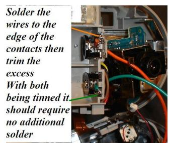
I solder the wires to the top edge of the battery contacts then cut the excess wire off and adjust the wires as tight and close to allow movement in the spring of the battery contacts.
