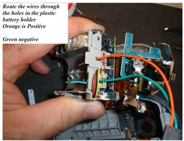
Slide the wires through the holes in the cameras plastic frame
