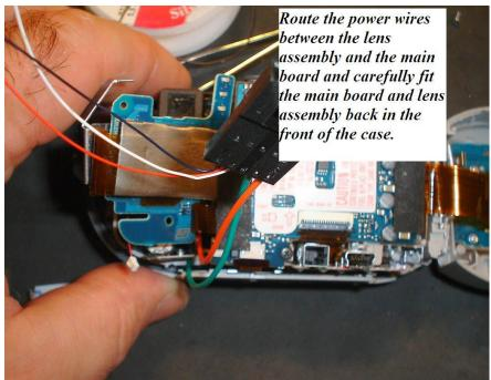
Flip the main board back into the front section it takes a little jogging and positioning to get the main board and the lens assembly back into place
