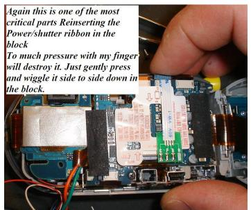
Gently use your finger to press the ribbon back into the block. If you would use too much pressure you will destroy the fragile contacts in the cable use a wiggling motion side to side pressure to gently get the cable seated.
