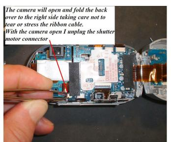
To open the camera pry it open and fold the back over to the right side Taking care not to pull or twist the ribbon cable
