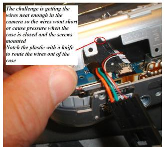
Now you need to close the camera up. Getting the wires as flat and smooth to the cameras main circuit board is important and this will allow it to close tightly without pinching any wires. I cut a small notch in the cameras back for the wires to get out of the camera. I secure the servo connector to the bottom of the camera with pt1100 tape and seal the holes and protect the wires with a dab of goop.
