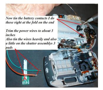
First heat the solder iron and tin both the wires and the battery contacts in the camera as shown Also apply a small amount of solder on the solder pads on the Hagshouse shutter assembly.
