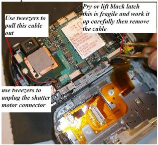
Once the camera is opened lift the tape off the backs cable lift the black latch carefully and slide cable out .There is a small cable on the top left side that also needs to be taken out Use tweezers and slide it out. Last is the shutter cover motor connector it easily unplugs with tweezers.
