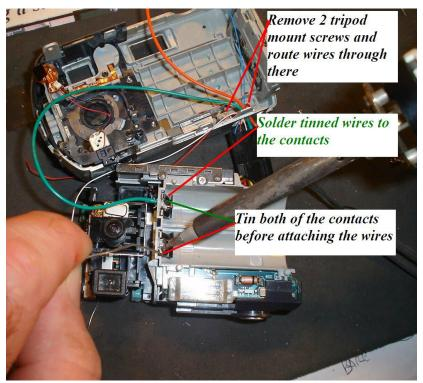
First tin the wires heavily and also tin the solder contacts on the camera Slide the wires through the holes we drilled and attach them by holding them tight to the contact then touch the hot iron to the contact No additional solder is needed or much heat if both the wire and contact were tinned first
