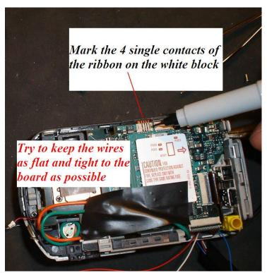
Tape the wires flat to the board and tuck what excess you can in the shutter motor hole. I then mark the 4 single contacts of the power/shutter block cable with a sharpie. Then remove the cable from the block by wiggling the cable out Try to not pull on the cable but lift it out by the ears many power cables are ruined by rough treatment of this cable.
