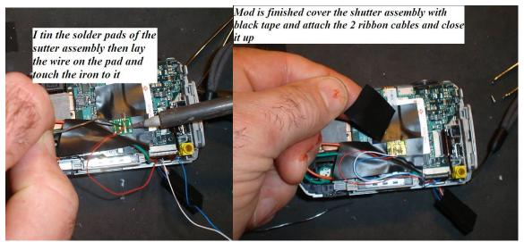
I will tin the pads then lay the wires on the shutter assembly and touch the hot solder iron to the pad Cover this with electrical tape after you are finished Attach the 2 ribbon cables and close the case halves reinsert the 4 screws and the camera should be fully operable it is best to test the working now before the sensor board is attached
