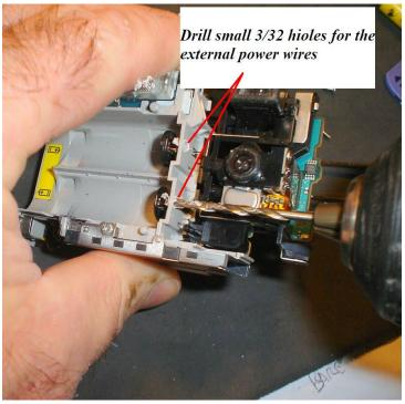
I find drilling a small 3/32" hole through the plastic case at the shown points is a great way to route the wires. This also acts as a holder so they won't get pulled or yanked easily.
