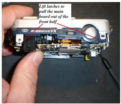
There are 2 small catches that hold the main board to the cameras front half
