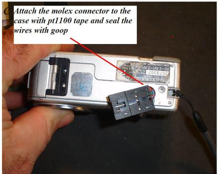
I use pt1100 tape to hold the Molex connector to the case and goop to cover and protect the wires where they come through the tripod mount.
