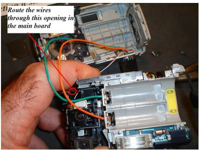
I then route the wires through the opening under or in this picture above the lens assembly
