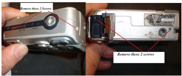
To open the camera 4 screws must be removed
