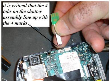
There are 4 metal contacts on the <u>www.hagshouse.com</u> shutter assembly Slide it in the empty white block lining the contacts with the marks we have made. Fold it over at a neat straight angle so the contacts won't shift then tape it down with black tape.
