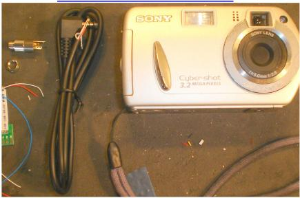
Parts required P32 camera Hagshouse shutter assembly 3 wire stereo plug kit Black tape
