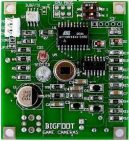
On the back side of the controller is your solderless camera connection plug and DIP switches that let you choose from four camera types, (or modes of operation where applicable). Here you also find, the PIR motion sensor, the day/night photocell and walk test LED. Also shown are jumper pads that will allow Bigfoot to work with many camera types, including all the newest ones.
