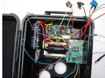
Now we can begin to connect the wires together. Good solder joints are a must as is covering the joints with electrical tape or Heat shrink tubing. Also I recommended using the 0.47 ohms resistor for four NiMH or alkaline cells and to get a 1.0 to 1.2 ohms for a 6-volt gel-cell.
