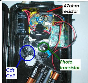
Now we are left to mount the Switch and the battery holder I use a piece of PVC board and attach it to the flash capacitor on the left side with pt1100 tape and on the right side I attach a piece of small plastic angle stock to the case then attach the board to it with PT1100 Tape also. In doing my builds this way I feel it makes a very neat finish with no holes drilled in the case other than the flash hole.
