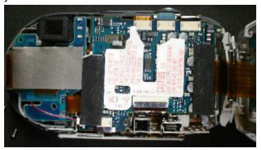
4. If you are using the stereo cable, then this is a good time to remove plastic out of the inside of the camera to make room for the jack. The circuit comes partially out of the front cover without having to remove anything extra, just be careful not to force it, because there is a ribbon cable and the wires to the lens cover motor attached to the bottom. Using a pair of side cutters, make the two cuts shown below.
