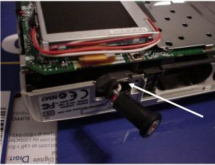
2. Disassemble the camera. There are seven screws that need to be removed.
