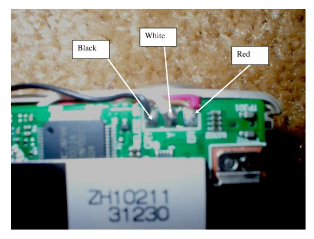
6. Mount the stereo jack into the tripod hole and let it dry and your done. Black is common (ground) = "G" on board White is Shutter = "S" on board Red is Refresh = = "O" on board
