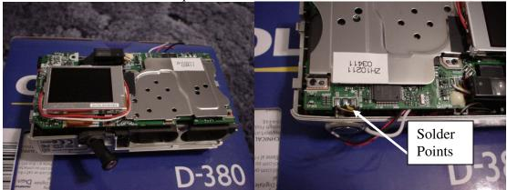
5. Solder the wires as shown and reassemble the camera.
